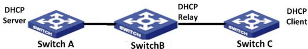
Figure 306 DHCP typical configuration example
