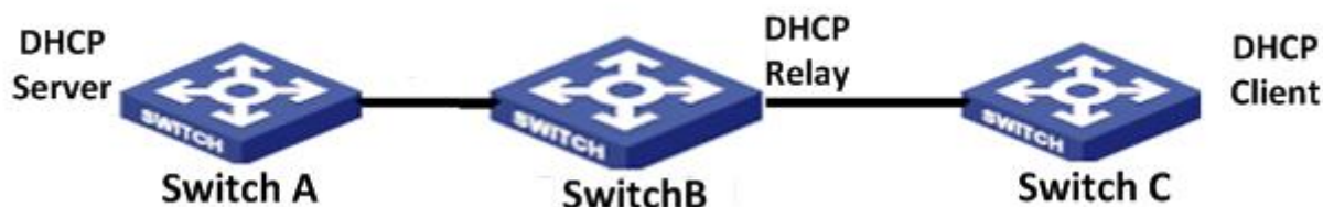
Figure 203 DHCP typical configuration example
