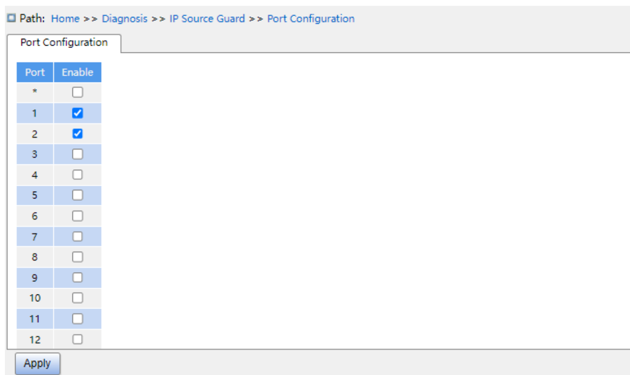
Figure 246 Configure Port IP Source Guard
